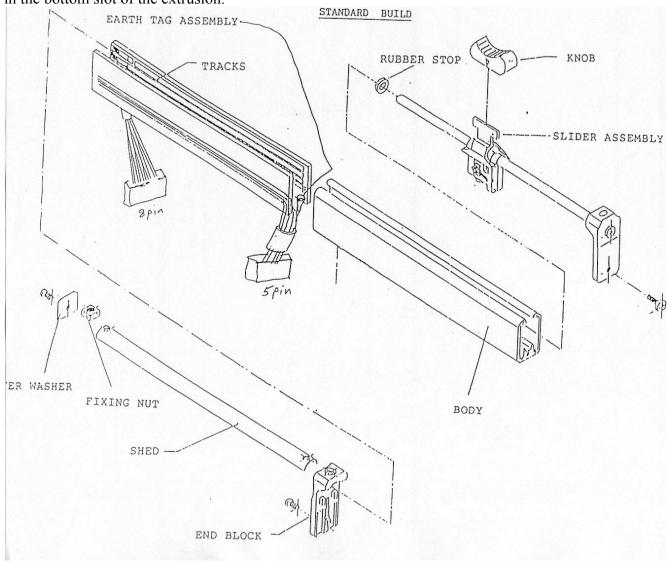
The long rectangular resistive tracks slide into slots along the inside of the extrusion. Simple mono faders utilize only one track, while more complicated faders such as stereo or motorized faders may contain tracks on both sides.
